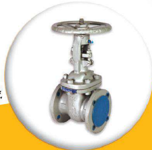
Gate/ Globe Valve CS, SS Body: WCB Size: From 2" to 36" Ratings: From 150# to 2500# Material: Forge Steel A-105N, Low Carbon Steel A216, WCB, WCC, WC6, WC9, A-351, CFB, CF8M, CF8C, CF3M, Duplex Steel
