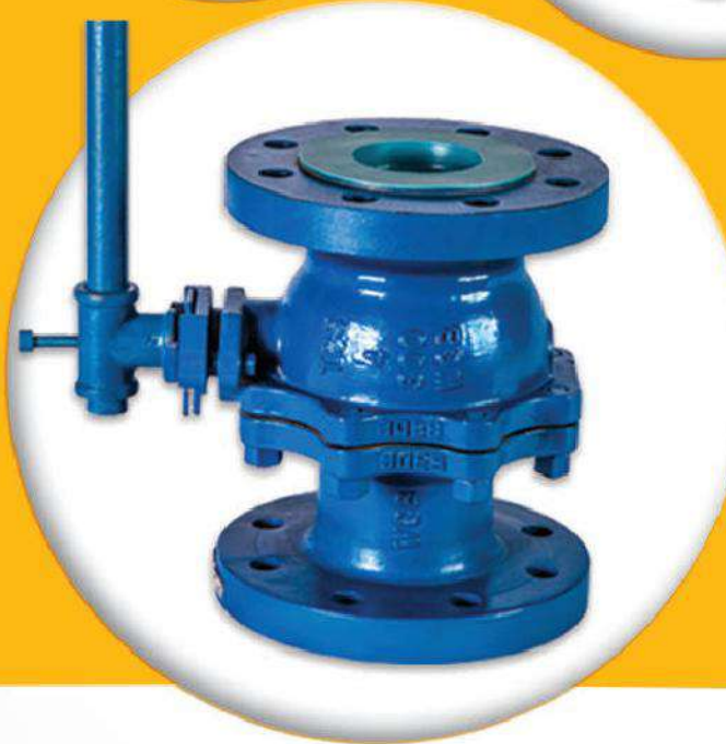
CS Ball Valve Body: WCB, A-105 Size: From 2" to 16" and 2" to 36" Ratings: From 150# to 2500#
